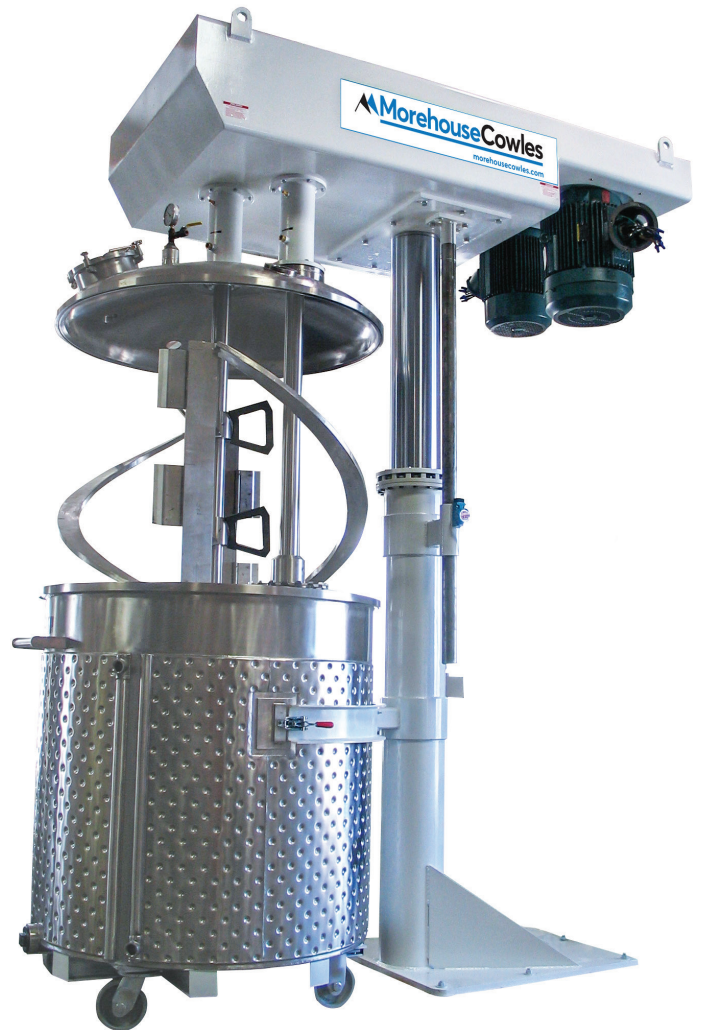
VISCOMAX™ MULTI-SHAFT MIXER: A multi-shaft dissolver is ideal for highly viscous products. The addition of wall scrapers on the sides and bottom of the anchor shaft ensures complete mixing. A third shaft is usually fitted with a screw-type auger, a tuning-fork-shaped gate blade or an axial flow-inducing turbine to minimize stratification and dead spots.
