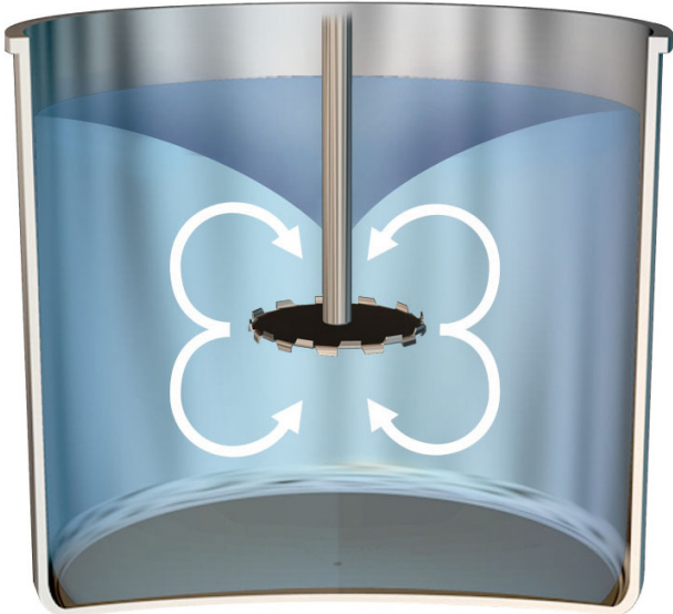
FIGURE 4: Causes laminar flow for "total motion"
