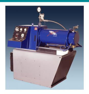
Patented Technology is used in this completely sealed, self-contained grinding and dispersion mill to produce superior fine and ultra-fine dispersions. The Zinger uses an exclusive rotor and vessel design to aggressively accelerate media. This patented design requires less energy and allows the use of smallre media to do the work. Low to extremely high viscosity slurries are easily and efficiently processed, using a unique rotor and chamber design.
