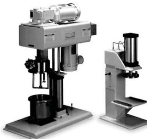
Every ViscoMax features at least two shafts to disperse material evenly throughout each batch. A high-speed impeller swirls ingredients throughout the tank. While a second, low-speed anchor blade wipes the vessel walls, pushing product continuously back into the high-shear zones for thorough dispersion and mixing.
